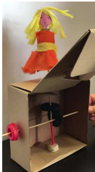
Figure 19: The Dancing doll uses a friction driver
