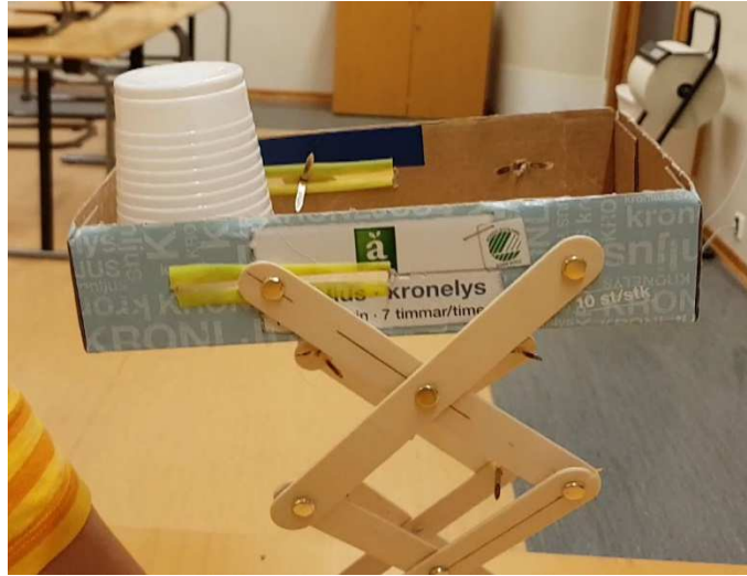
Figure 15: The scissor lift uses a slider linkage
