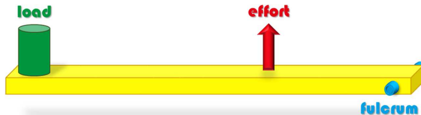
Figure 8: A type 3 lever
